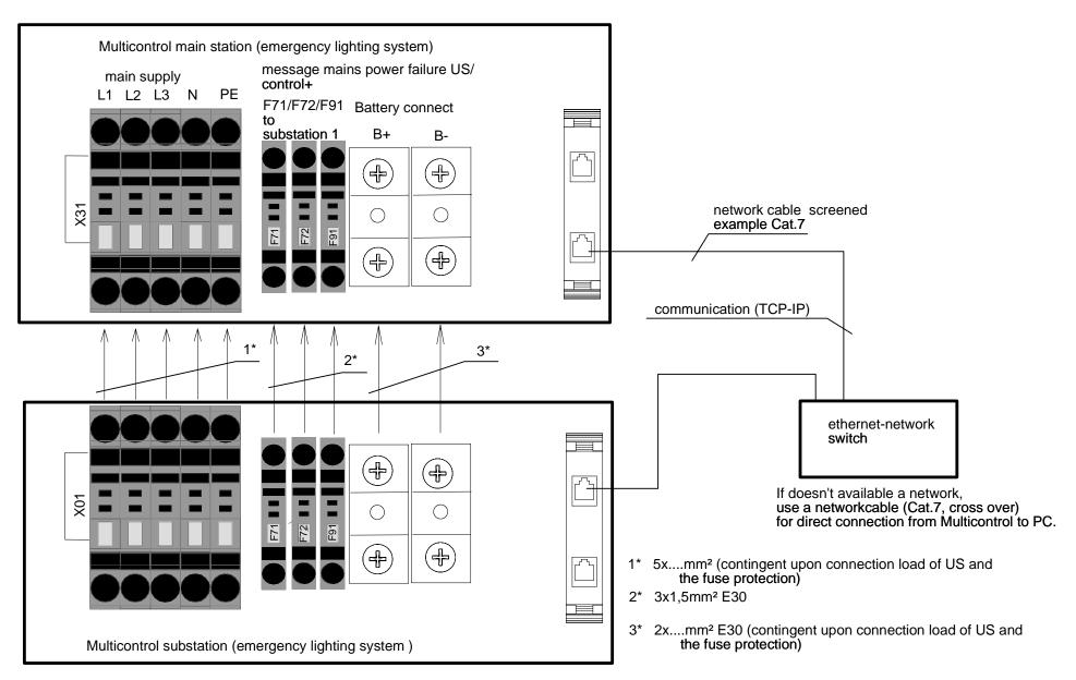
For a faultless function you must connect all wire !
