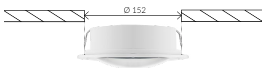
zestaw do montażu wpuszczanego option with recessed mount kit applied
